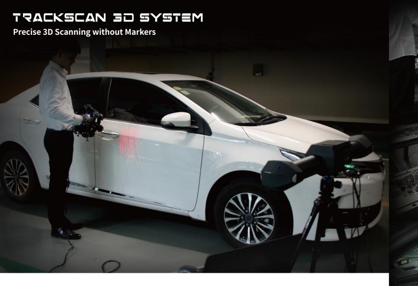
TrackScan 3D system delivers high-precision 3D solution without markers. In combination with 3D laser scanning technology and flexible probing function, it offers rapid and accurate data collection of overall size and key features.
